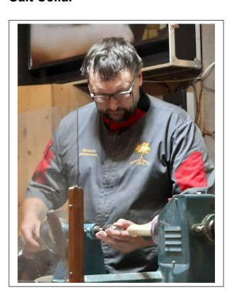
After break Gintaras made a salt cellar using an apple wood blank approximately 110 – 130mm X 60 – 70mm. The blank was mounted between centres and trued with a tenon. After being mounted in a chuck the end of the blank was trued and a hole drilled 20mm x 55mm deep with a Forstner bit. Then the blank was marked at 65mm and the measurement cut in to establish the
