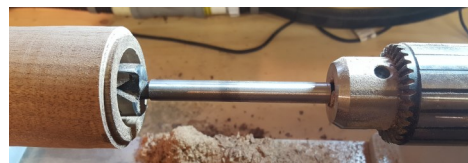
5. Main body with 300mm forstner bit & extension bar
