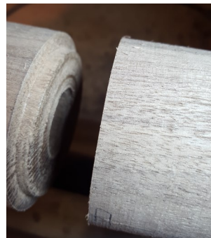
10. Main body fitting the spigot of head
