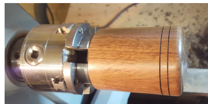
14. Finishing head on chuck
