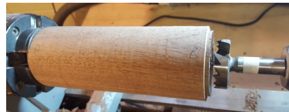
3. Main body with marked 45mm forstner bit
