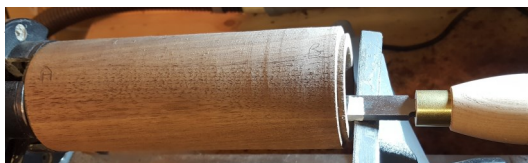
6. Offset tool marked to 46mm
