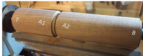
2. Stock turned round, spigots & marked
