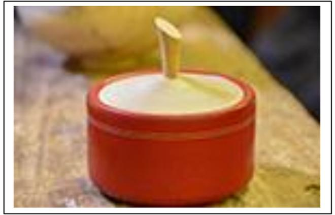
After scraping the inside a recess was cut for the lid and the top and bottom of the blank were gently rounded over. At this stage Robert used 'Holiday Red' milk paint by General Finishes ([Here](#)) to cover the outside of the box. It was applied with a sponge brush in two or three layers but it still allows the grain to show through. No sealer is necessary and the paint can be covered with acrylic lacquer ([Gloss Lacquer](#)) to finish.
