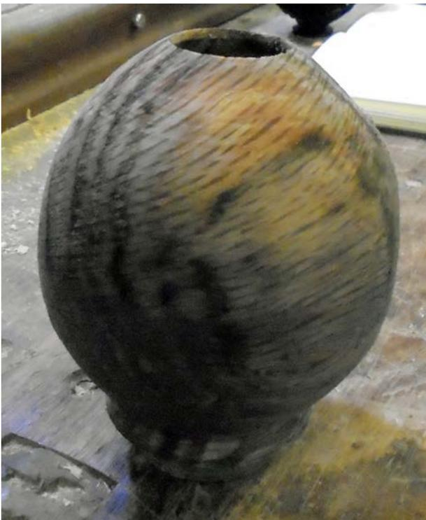
turned and stored in a vat of water so that the wood will move easily when turned on the lathe.
