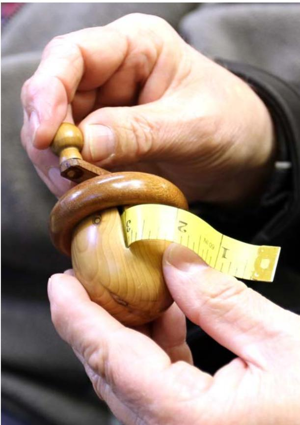
is made by drilling a 6mm hole in the blank and shaping the knob to whatever style you wish. It can be parted off and finished by hand or you could make a 6mm tenon and mount the knob on that to do the tidy-up work and sanding etc.
