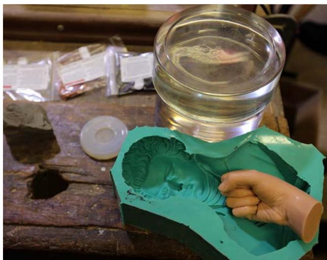
When using silicon rubber you need to be careful to avoid moisture while the mould is setting and Fast Cast Polyurethane will set in about 15 minutes so you will get results quite quickly. The type of material you use for the mould will depend on the desired result e.g. if you want to lift a lot of detail use a soft silicon mould material. It is advisable to use some sort of mould release to ease extraction of the cast. This could be wax, silicon or spray teflon.
