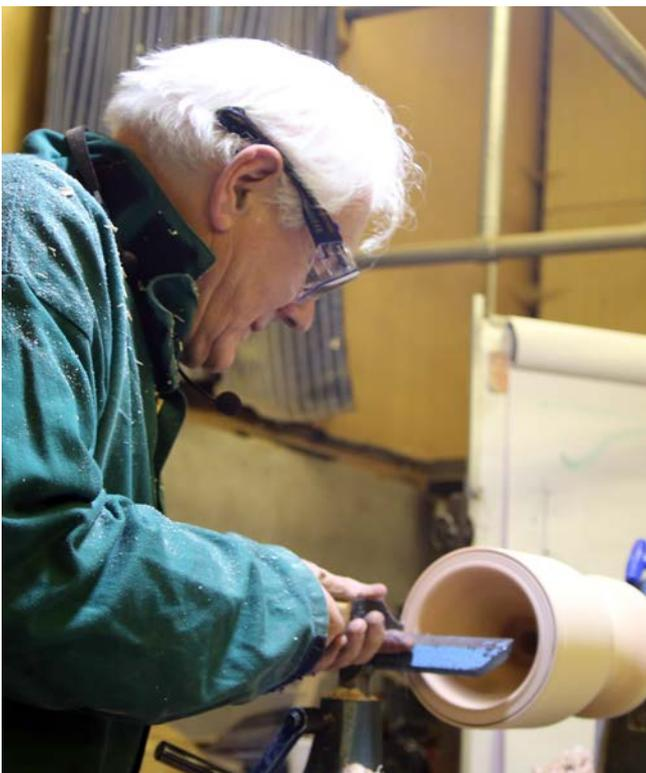
a hacksaw blade. Made some fine adjustments then shaped the outside of the vessel.
