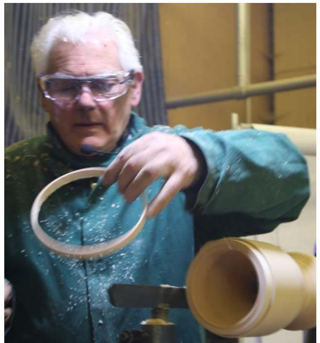
Danny then refined the outside of the vessel, shaped the bottom. He made the outside in an elliptical shape, showing us how to draw an ellipse using a clever little jig he had made. He then cut out the lips from the drawing and used that to refine his shape.
